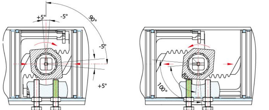
Standard stroke:  $0^\circ \pm 5^\circ \sim 90^\circ \pm 5^\circ$
