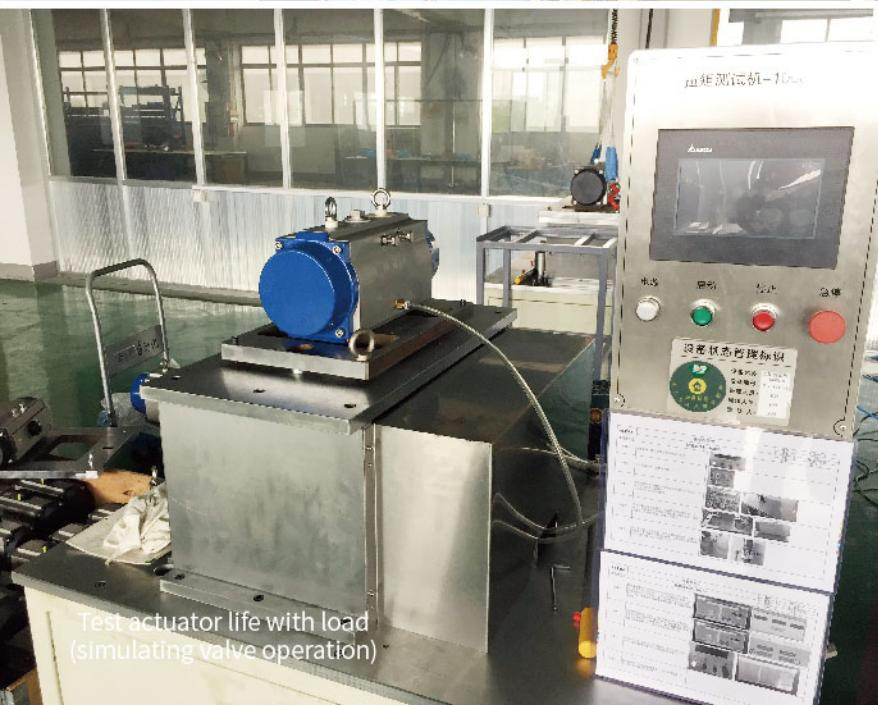
Test actuator life with load
